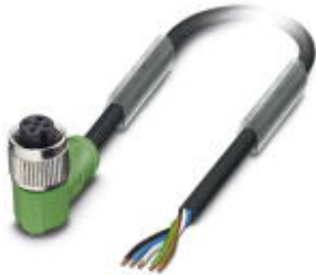
Sensor/Actuator cable, 5-position, PUR halogen-free, Black-gray RAL 7021, Free cable end, on Socket angled M12, A-coded, Cable length: 10 m
