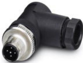
Sensor/actuator connector, male, angled, 5-pos., M12, A-coded, screw connection, metal knurl, cable screw connection Pg9
