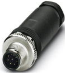
Sensor/actuator connector, male, straight, 8-pos., M12, A-coded, screw connection, metal knurl, cable screw connection Pg9
