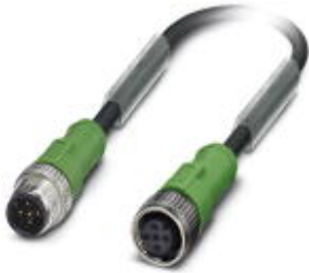
Sensor/Actuator cable, 5-position, PUR halogen-free, Black-gray RAL 7021, Plug straight M12, A-coded, on Socket straight M12, A-coded, Cable length: 0.6 m
