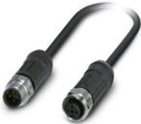
Sensor/Actuator cable, 4-position, PE-X halogen-free, Black-gray RAL 7021, Plug straight M12, A-coded, on Socket straight M12, A-coded, Cable length: 5 m, For outdoor applications, With high-grade steel knurl
