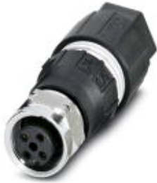
Sensor/actuator connector, Universal, 4-position, Plug straight M12, A-coded, Insulation displacement connection, Knurl material: High-grade steel, External cable diameter 4 mm ... 8 mm
