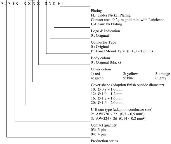
373: Mini Clamp Wiremount Socket Connector
