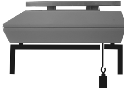
Fig. 1: Setup of balance for underfloor weighing
