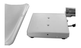
1. Push the front of the weighing pan (arrow) up to the stop across the weighing platform.
