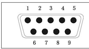
Pin 2: TXD - Output Pin 3: RXD - Input
