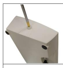
Take a screw driver and remove the plastic covers from both sides of the display unit.
