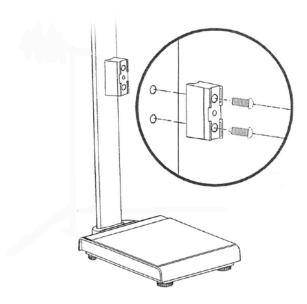
Use the 2 screws for screwing the bracket into the supplied insert nuts on the stand of the scales.
