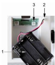
Carefully insert the rechargeable battery block and insert plug into connection CN 3
