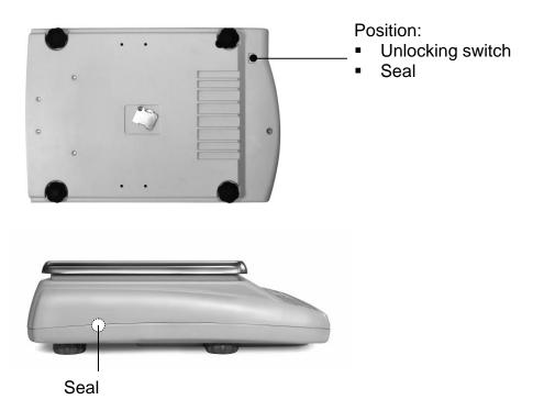
After verification the balance is sealed at the indicated positions. **Verification of the balance is invalid without the "seal".**
