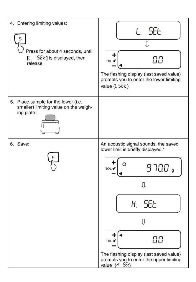
7. Place sample for the upper (i.e. larger) limiting value on the weighing plate:
