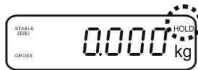
⇒ Place the load onto the weighing system and wait until it is fairly stable.
