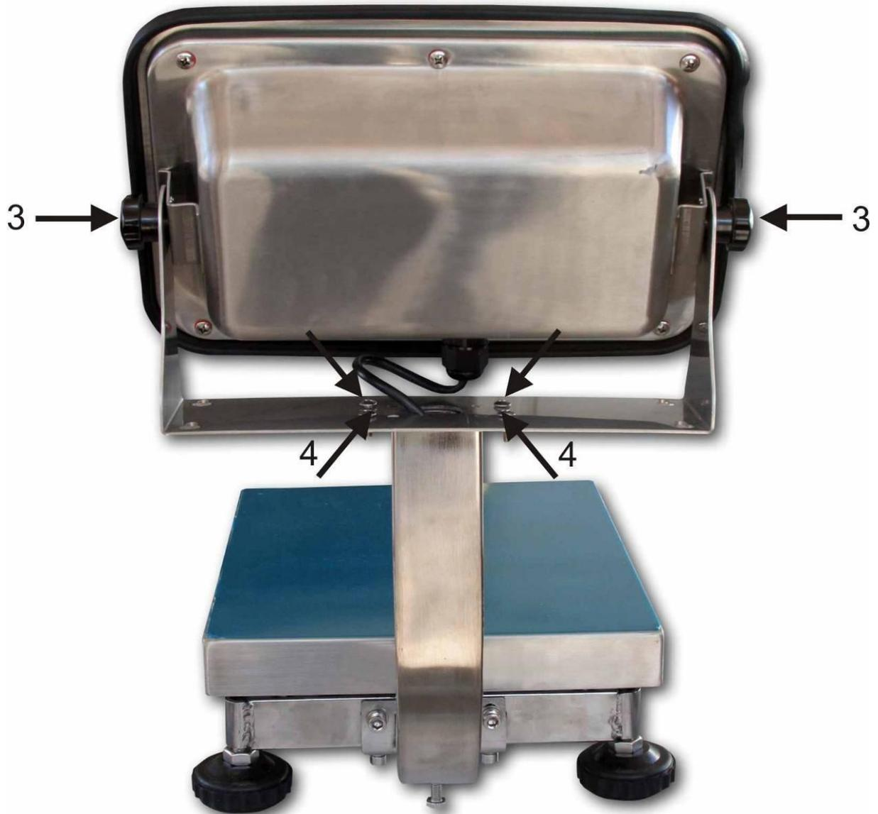
Attach the tripod with the four raised counter-sunk head screws [4] and the nuts on the holder of the display unit.
