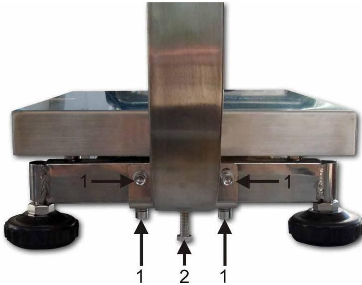
Attach the tripod to the platform acc. to fig. using the 4 screws [1], securing disks and washers. Ensure that the cable is not damaged nor squeezed. Screw-in support screw [2] till it is safely fixed.
