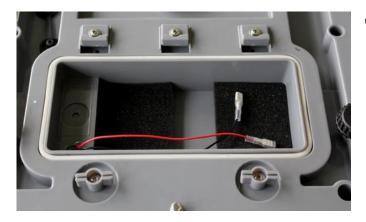
⇒ Remove battery compartment cover and the foam pieces
