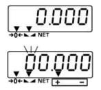
⇒ In weighing mode press for about 3 seconds, the display for entering the upper limit appears. The left digit blinks. A triangle appears above the "+" symbol. Moreover, the background of the screen turns red.
