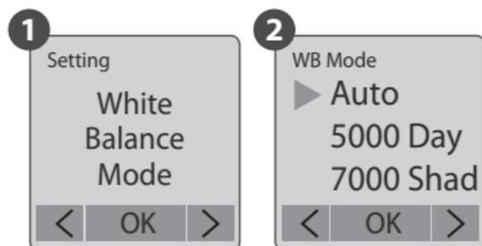
At the default setting of Auto (AWB), the camera automatically adjusts white balance so that a white subject will appear white regardless of the color of the light source. It may however be necessary to match white balance to the light source under mixed lighting or when photographing a subject that is a solid color.
