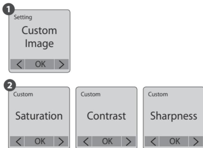
Control Saturation, Contrast, Sharpness. Select and enter each setting, using **MENU** (←) and **TIME** (→) to adjust the effect. Then press **OK** to exit.
