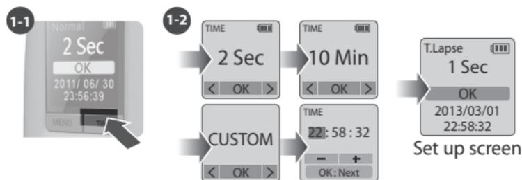
1-1 Press **TIME** button to enter time interval set up.
