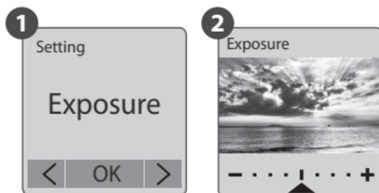
In the Exposure setting menu, press **MENU** (→) to increase (+) exposure time or select **TIME** (←) to decrease (-) the exposure time. Press **OK** to exit.
