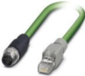
Assembled PROFINET cable, CAT5e, shielded, star quad, AWG 22 stranded (7-wire), RAL 6018 (yellow-green), M12 plug to RJ45 plug/IP20, line, length: 3 m
