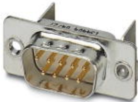
D-SUB contact insert, shell size 1, with nine signal contacts, contact type pin, for PCB assembly, angled, fixing with a 2.5 mm hole and solder metal plate, for panel mounting frame VS-09-...
