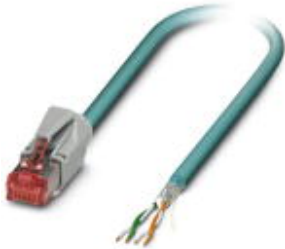
Assembled Ethernet cable, CAT5e, shielded, 2-pair, 26 AWG stranded (7-wire), RAL 5021 (water blue), RJ45 plug/IP20 to free cable end, line, length: 2 m
