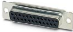
D-SUB contact insert, shell size 3, with 25 signal contacts, contact type socket, with solder cup, straight, fixing with a 3 mm hole, for panel mounting frame and sleeve housing VS-25-...
