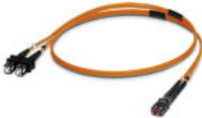
Assembled FO cable, break out cable, multi-mode fiberglass 50/125 µm, connector: SC Duplex / SCRJ, protection type: IP20, for installation in cable ducts or control cabinets, length: 2 m ^
