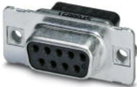
D-SUB contact carrier, shell size 1, for nine signal contacts, contact type socket, for crimp contacts, straight, fixing with 4-40 UNC thread, for panel mounting frame VS-09-...
