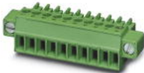
Plug component, Nominal current: 8 A, Rated voltage (III/2): 160 V, Number of positions: 12, Pitch: 3.81 mm, Connection method: Screw connection, Color: green, Contact surface: Tin
