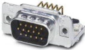
D-SUB contact insert, shell size 1, with 15 signal contacts, contact type pin, for PCB assembly, angled, fixing with 4-40 UNC thread and solder pins, for panel mounting frame VS-09-...
