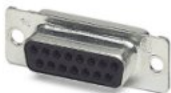
D-SUB contact insert, shell size 2, with 15 signal contacts, contact type socket, with solder cup, straight, fixing with a 3 mm hole, for panel mounting frame and sleeve housing VS-15-...
