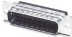
D-SUB contact carrier, shell size 3, for 44 signal contacts, contact type pin, for crimp contacts, straight, fixing with a 3 mm hole, for panel mounting frame and sleeve housing VS-25-...
