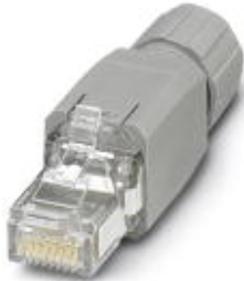
RJ45 connector, IP20, CAT5e, 4-pos., PROFINET with QUICKON fast connection technology, for 1-wire and 7-wire conductors AWG 22, for cable diameter 4.5 mm ... 8.0 mm, color: gray
