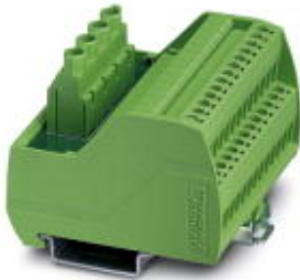
VARIOFACE module, with two equipotential busbars (P1, P2) for potential distribution, for mounting on NS 35 rails. Module width: 90.8 mm
