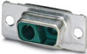
D-SUB contact carrier, shell size 1, accommodation for two combined contacts, contact type socket, straight, fixing with a 3 mm hole, for panel mounting frame and sleeve housing VS-09-...
