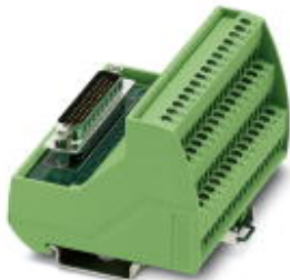
VARIOFACE module, with screw connection and high density D-SUB miniature socket strip, for mounting on NS 35 rails, no. of pos.: 26, width: 79 mm
