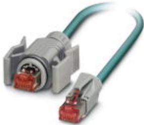
Assembled Ethernet cable, CAT5e, shielded, 2-pair, 26 AWG stranded (7-wire), RAL 5021 (water blue), RJ45 plug/IP67, gray to RJ45 plug/IP20, line, length: 1.5 m
