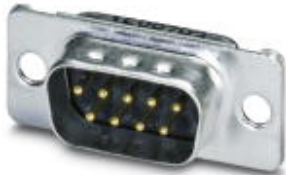
D-SUB contact insert, shell size 1, with nine signal contacts, contact type pin, with solder cup, straight, fixing with a 3 mm hole, for panel mounting frame and sleeve housing VS-09-...
