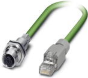
Assembled PROFINET cable, type B, CAT5e, shielded, star quad, AWG 22 stranded (7-wire), RAL 6018 (yellow-green), panel feed-through, M12, 4 pos., D-coded on RJ45 connector, length: 0.5 m
