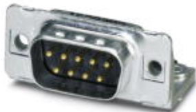
D-SUB contact insert, shell size 1, with 9 signal contacts, contact type pin, for PCB mounting, angled, fixing with M3 thread and solder pins, for panel mounting frame VS-09-...
