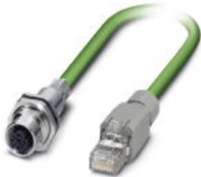
Assembled PROFINET cable, type B, CAT5e, shielded, star quad, AWG 22 stranded (7-wire), RAL 6018 (yellow-green), panel feed-through, M12, 4 pos., D-coded on RJ45 connector, length: 1 m
