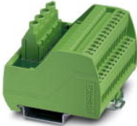
VARIOFACE module, with two equipotential busbars (P1, P2) for potential distribution, for mounting on NS 35 rails. Module width: 70.4 mm
