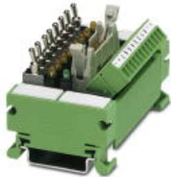
VARIOFACE switch module, with flat-ribbon cable and COMBICON connector, for simulation, for 8 signals, for mounting on NS 35/7.5
