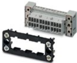
Contact insert set for mounting side, sleeve frame with PE, 4 fixing screws, 8-pos. contact inserts preassembled, 6 coding profiles, 2 mounting flanges
