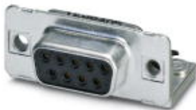
D-SUB contact insert, shell size 1, with 9 signal contacts, contact type socket, for PCB mounting, angled, fixing with M3 thread and solder pins, for panel mounting frame VS-09-...
