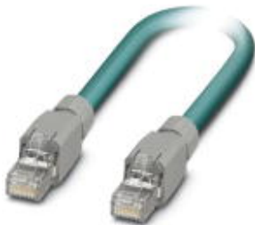
Assembled Ethernet cable, shielded, 4-pair, 26 AWG suitable for use with drag chain (19-wire), RAL 5021 (water blue), RJ45 plug/IP20 to RJ45 plug/IP20, line, length: 10 m
