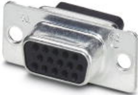
D-SUB contact carrier, shell size 1, for 15 signal contacts, contact type socket, for crimp contacts, straight, fixing with a 3 mm hole, for panel mounting frame and sleeve housing VS-09-...
