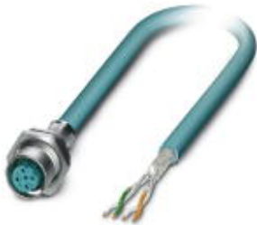
Assembled Ethernet cable, CAT5e, shielded, 2-pair, AWG 26 stranded (7-wire), RAL 5021 (water blue), M12 flush-type socket, rear/screw mounting with M16 thread on free conductor end, line, length 2 m
