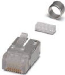
RJ45 pin insert, CAT5e, 8-pos., shielded, IDC connection method, for litz wires AWG 26 and solid wires AWG 26 ... 24
