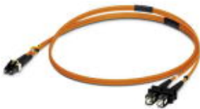
Assembled FO cable, break out cable, multi-mode fiberglass 50/125 µm, plug: LC / SC-Duplex, protection type: IP20, for installation in cable ducts or control cabinets, length: 5 m
