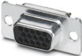
D-SUB contact insert, shell size 1, with 15 signal contacts, contact type socket, with solder cup, straight, fixing with a 3 mm hole, for panel mounting frame VS-09-...
