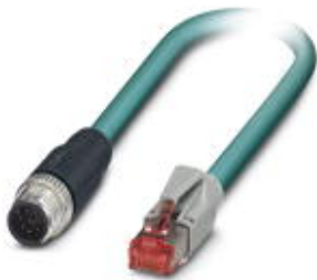
Assembled Ethernet cable, shielded, 4-pair, 26 AWG stranded (7-wire), RAL 5021 (water blue), M12 plug to RJ45 plug/IP20, line, length 3 m
