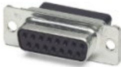
D-SUB contact carrier, shell size 2, for 15 signal contacts, contact type socket, for crimp contacts, straight, fixing with 4-40 UNC thread, for panel mounting frame VS-15-...
