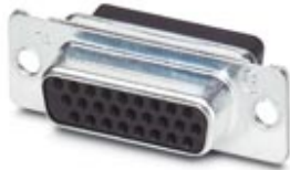
D-SUB contact carrier, shell size 2, for 26 signal contacts, contact type socket, for crimp contacts, straight, fixing with a 3 mm hole, for panel mounting frame and sleeve housing VS-15-...
