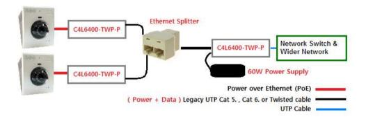
C4L6400-TWP-P transceivers are used to extend the Ethernet IP signals via Cat 5E, Cat 6 or 2 wire cable in the existing UTP network in building.
