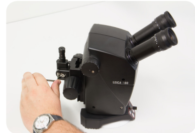
Open the two screws on the focus arm of the Leica A60...
