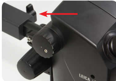
Attach Leica A60 to flex arm and tighten knob to secure the instrument.
