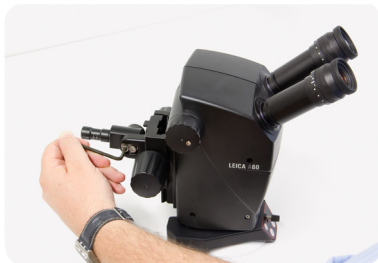
...and bring pin into horizontal position. Tighten screws again.
