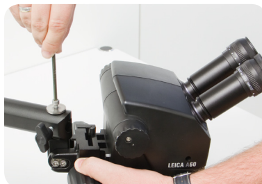
... and immediately secure the instrument with previously removed washer and screw.
