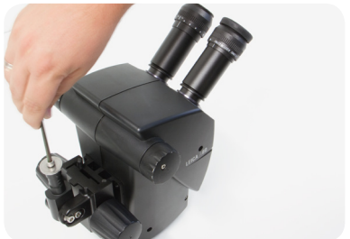
Remove allen screw and washer from the Leica A60 instrument as shown.
