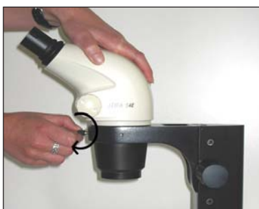
Fix StereoZoom® with clamping screw by turning screw clockwise
